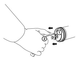
Take particular care that all surfaces are cleaned of grease and oil. Rinse and dry all parts thoroughly before reassembling them.
